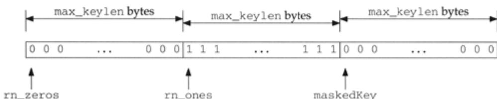
`rn_zeros` is an array of all zero bits, `rn_ones` is an array of all one bits, and `maskedKey` is an array used to hold a temporary copy of a search key that has been masked.
