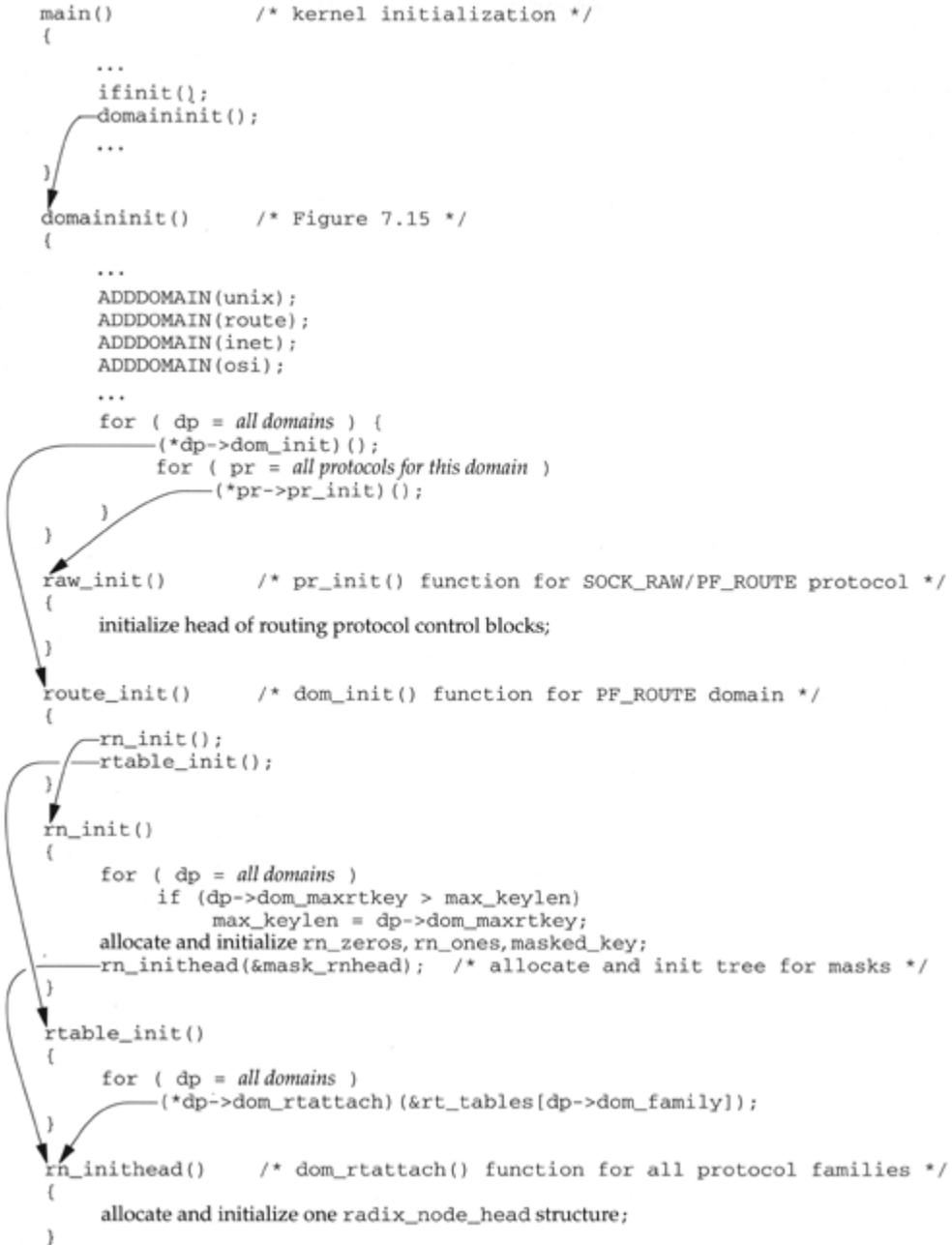
domaininit is called once by the kernel's main function when the system is initialized. The linked list of domain structures is built by the ADDDOMAIN macro and the linked list is traversed, calling each domain's **dom\_init** function, if defined. As we saw in Figure 18.27, the only dom\_init function is route\_init, which is shown in Figure 18.30.
