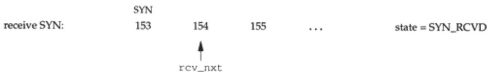
Figure 28.20 sets the TF\_ACKNOW flag and the segment generated by tcp\_output will contain a SYN and an ACK (the tcp\_outflags value in Figure 24.16). The sequence number of the SYN is 153 and the acknowledgment number is 154.
