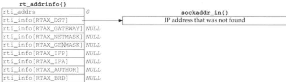
All the unused pointers are null because the structure is set to 0 before it is used. Also note that the `rti_addrs` member is not initialized with the appropriate bitmask because when this structure is used within the kernel, a null pointer in the `rti_info` array indicates a nonexistent socket address structure. The bitmask is needed only for messages between a process and the kernel.
